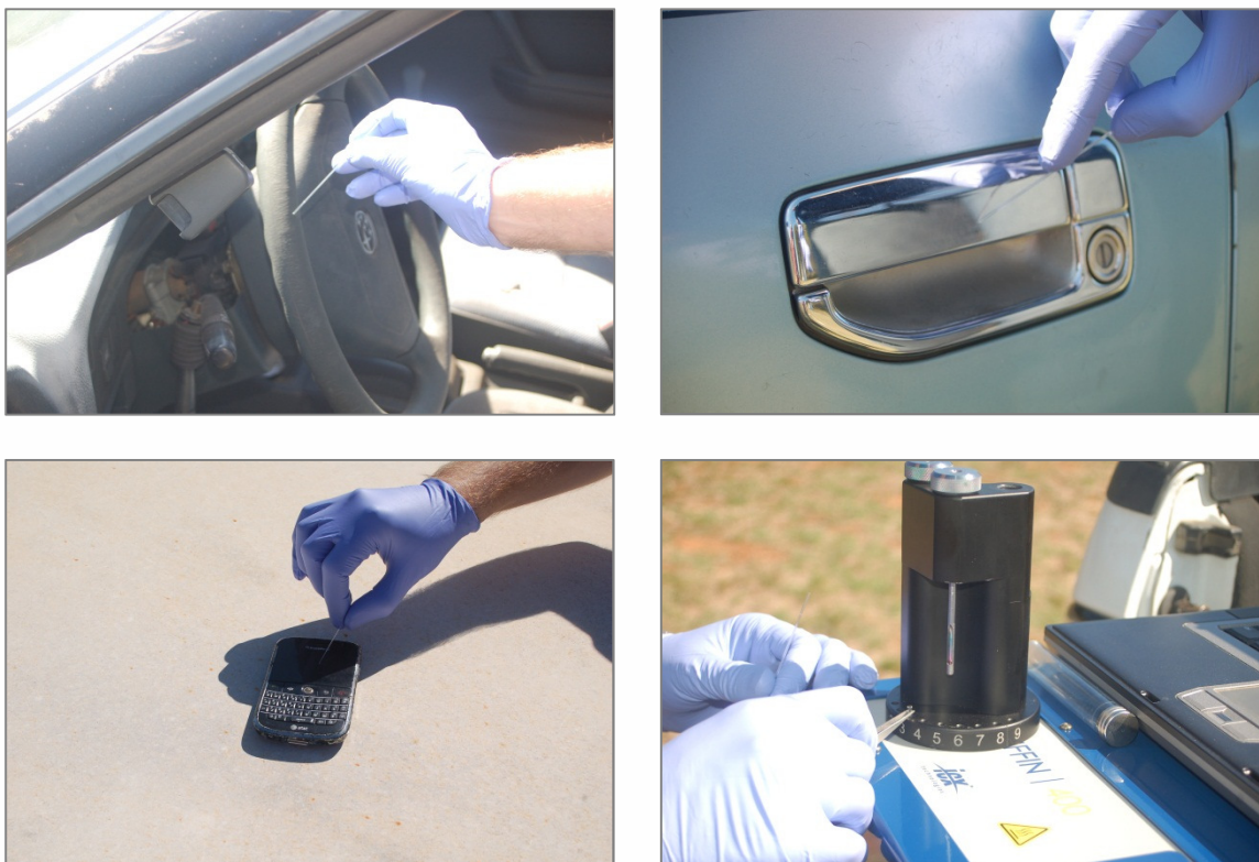
Figure 3: Sampling of explosive residue via TAG, with subsequent analysis by Griffin GC/MS.
