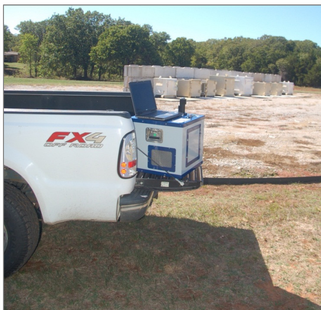
Figure 2: The rugged Griffin GC/MS operating at the FLIR explosive testing facility.
