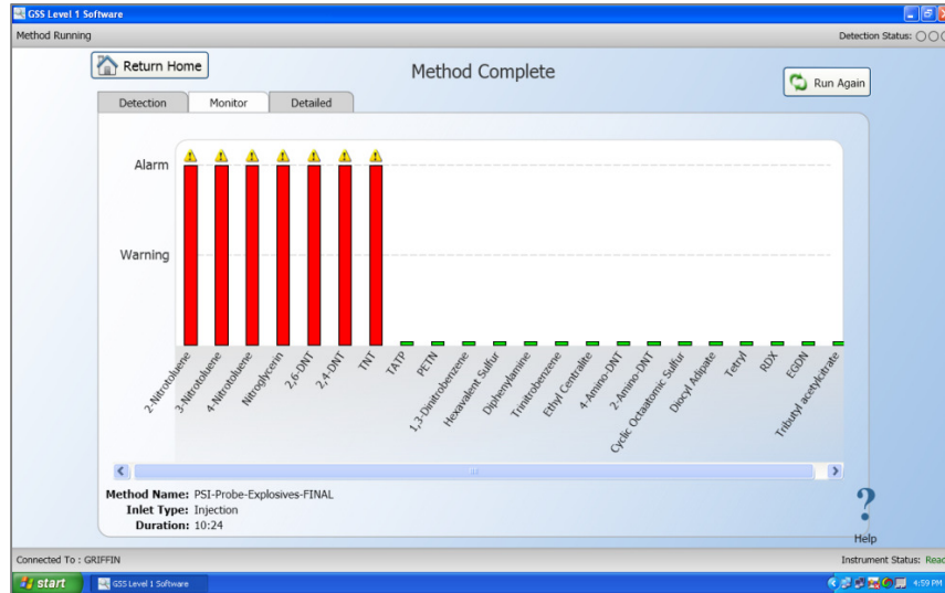
Figure 6: Real-Time Detection of Wabox Constituents displayed in GSS Level I.
